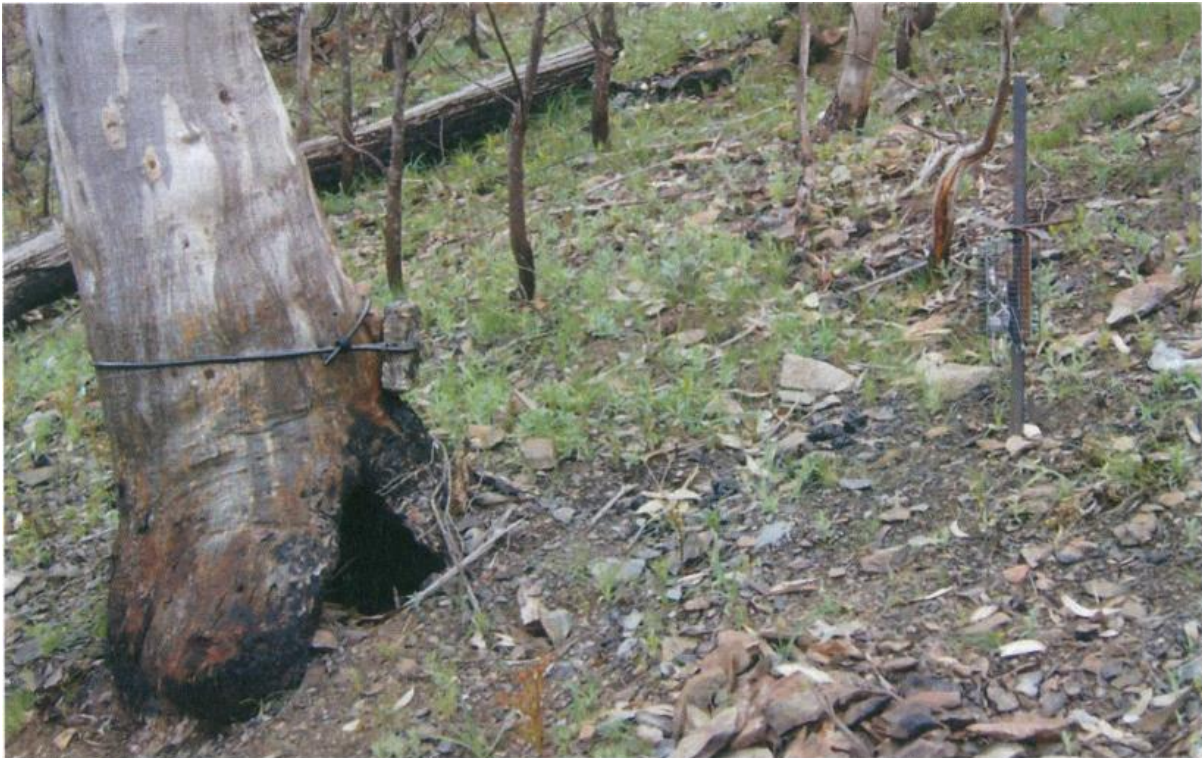
Figure 4: An example of a remote camera set opposite a bait station to detect small mammals. The unit is attached to the tree so the sensor is 20cm above the ground and approximately 1.5m from the bait station.
